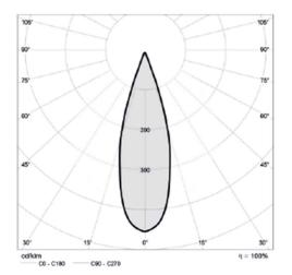
Correlated color temperature: 3000 – 6000 kelvin Rated median useful life: 50000h L70 at 25°C Luminaire input power: 7 w
